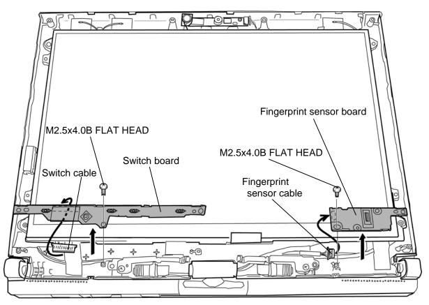
Figure 4-56 Removing the switch board/fingerprint sensor board
